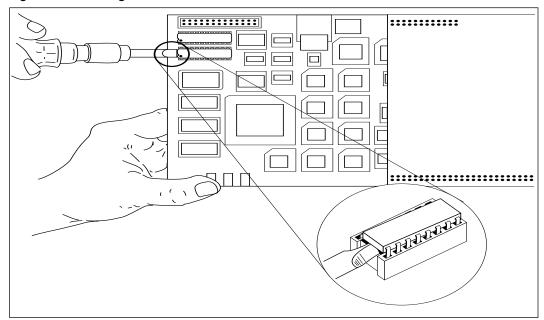
3. Remove both PEB terminators, XRN1 and XRN2, from any remaining DVCs.
